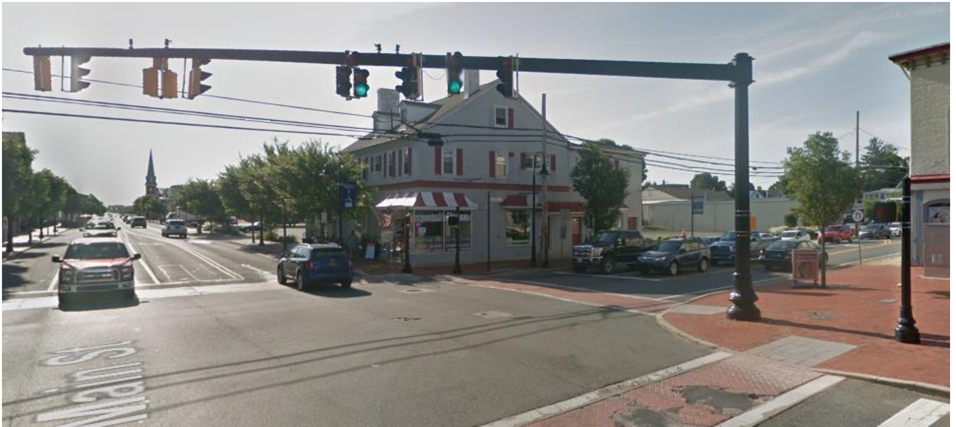
Main Street and Broad Street in Middletown. The poles shown are ornamental with the ornamental base.
